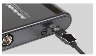
To receive broadcast TV signals, connect the included TV whip antenna to the RF (antenna) jack on the TV tuner.
